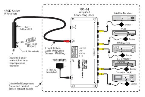
Since the IR receiver is in close proximity to the audio/video equipment, no wiring extension should be required so long as the connecting block is within reach of the 7-foot cable. The 3.5mm stereo type mini plug is connected to the "IR RCVR" jack on the Xantech Connecting Block.
